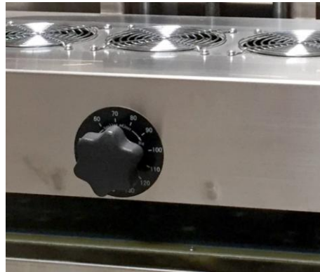
Figure 8. Adjust cap diameter guide based on sealing cap diameter
