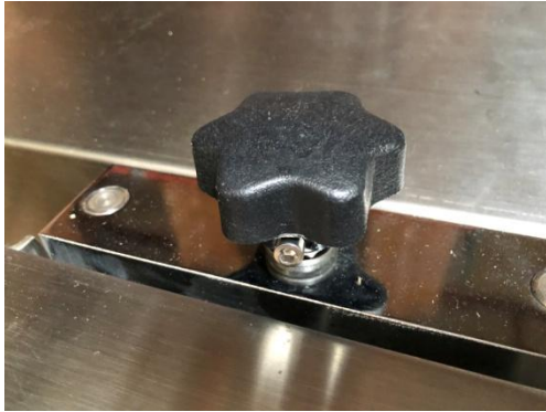
Figure 6. Knob to adjust the height of sealing container
