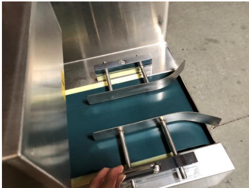
Figure 7. Adjust guides with allen wrench
