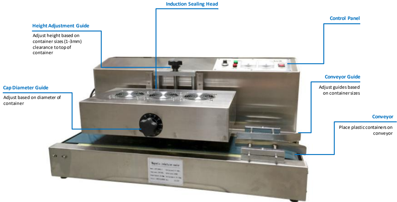
Figure 2. LGYF-Series Induction Sealer Overview
